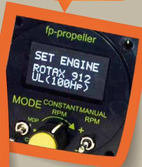
Core of the governor is a last generation CPU, operating with the engine constant RPM target. Embedded firmware acquires continuously data from sensors, process these data and decide on this basis. In order to do this job at high speed, firmware is splitted in blocks processed in multitasking.
