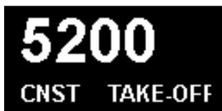
Once the 5000 RPM is exceeded and for 3 minutes (in the case of Rotax engines), the system adds an offset of +300 RPM to the TARGET RPM calculated by the system (MDP DRIVEN) or set by the pilot (CONSTANT RPM) so the engine can reach 5800 RPM for the take-off phase.
