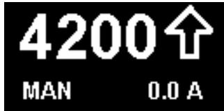
The display indicates **actual RPMs** and, during propeller motion, the power consumption of the servomotor of the propeller (Ampere), as a diagnostic of the correct functioning of the system.
