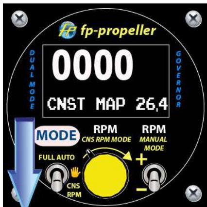
In this mode, the pilot decides the target RPM by turning the potentiometer (B) and the governor moves the propeller pitch to reach that target value. The Governor maintains that target value independently of the handle, within the limits set by the aircraft, the propeller and the flight conditions. The setting range for Rotax engines ranges from 4000 to 5500 RPM (4300 to 5800 RPM in takeoff mode, please check chapter 7 for other modes)
