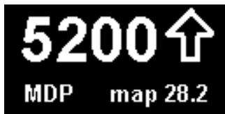
The value shown in the OLED display is the **TARGET RPM** value, the system has a hysteresis of  $\pm 100$  rpm to avoid unnecessary stresses on the propeller servomotor, so the actual RPM value may differ by  $\pm 100$  rpm
