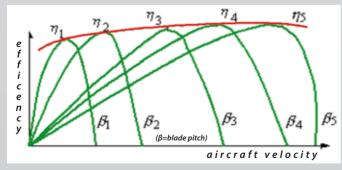
The use of the embedded characteristic diagrams of the engine, assure the achievement of the best efficiency of engine / propeller couple.
